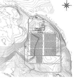
The project is focused on a waste treatment facility for the Sulaimaniyah Municipality ("Ecocem Iraq"). It includes a mechanical pre-treatment facility, a bio-drying unit, a dried waste sorting facility to separate inorganic (primarily inert waste streams) and organic (fuel value waste streams), and a landfill for the inert fraction to provide a complete waste management solution for the Sulaimaniyah Municipality. The work area occupies, approximately, 12 hectares.
